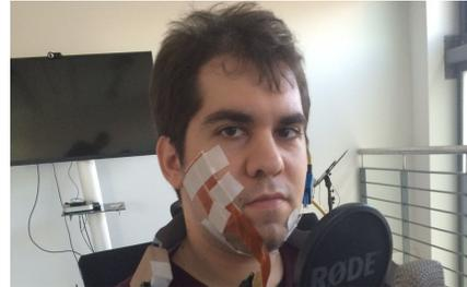
Fig. 1. Positioning of the electrodes, with one  $4 \times 8$  electrode array on the cheek and an 8 electrode strip below the chin.
