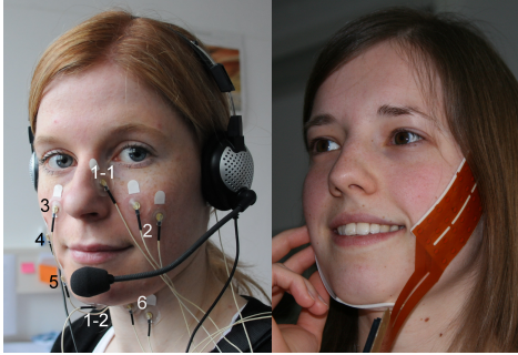
Figure 2: left: Single electrode positioning, black numbers indicate unipolar derivation with reference electrodes behind the mastoid bone (except channel 1), white numbers indicate bipolar derivation. right: Electrode array positioning, one large array is positioned on the cheek, one small array under the chin. See text for details.
