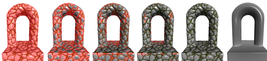
Figure 7.3: The first frames after a cache clear for a displaced and coloured arch. Cache misses are marked red. The untextured base model is shown on the very right.
