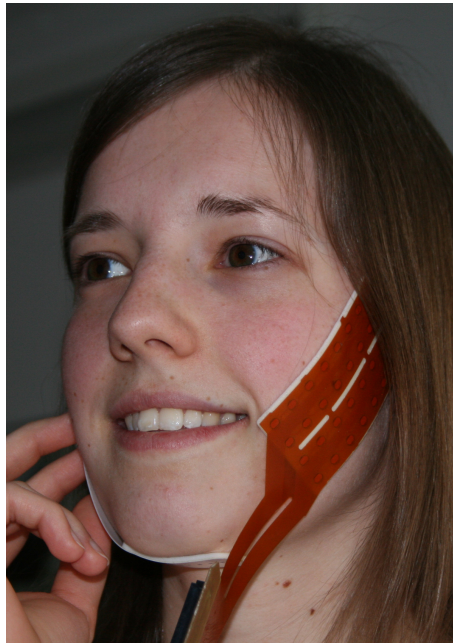
Figure 5.2: The array recording setup, with a 4x8 electrode array on the cheek and a smaller 1x8 electrode array under the chin.
