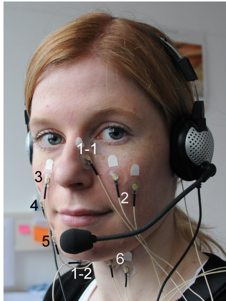
Figure 5.1: The single-electrodes recording setup, with electrode positions marked. White numbers indicate bipolar derivation, whereas black numbers indicate unipolar derivation against a reference electrode attached behind the ear.
