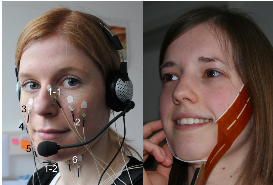
Fig. 2. left: Single electrode positioning, black numbers indicate unipolar derivation with reference electrodes behind the mastoid bone (except channel 1), white numbers indicate bipolar derivation. right: Electrode array positioning, one large array is positioned on the cheek, one small array under the chin. See text for details.
